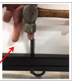
Slide the spring on the back side of the latch, then hold the retainer cap and ap on using a hammer
